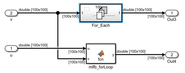
The For Each Subsystem contains a Gain block that executes 100 times. The MATLAB Function block contains code with a for-loops that performs element-wise operations:
