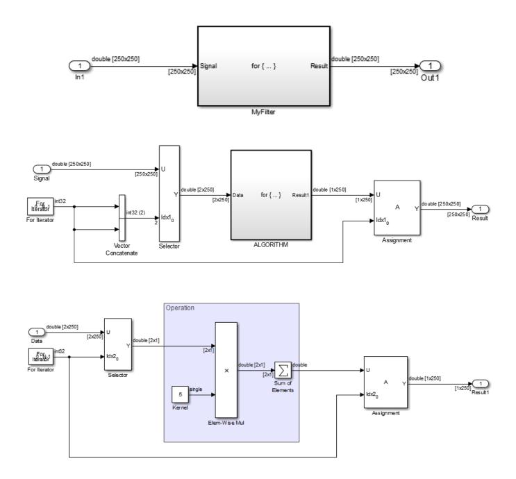
ALGORITHM, which is nested in MyFilter. Both subsystems contain a for Iterator block, a Selector block, and an Assignment block.
